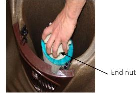
The spa's automatic surface skim filter is designed to remove floating debris and contaminants such as body lotions by drawing water through a specially formulated filter cartridge element. It is critical that this element be routinely cleaned.
