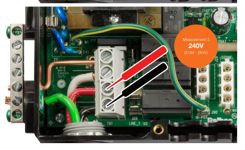
Measure voltage between the terminal block and fuse. The fuse is labeled F2 on the circuit board.
