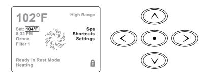
Navigational buttons serve for the purpose of selecting individual functions. A selected function is highlighted by a white outline and the text turns white. Once the function is selected, you can control it by pressing the middle button.
